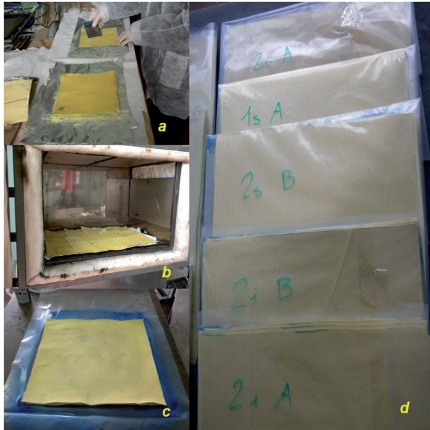
Figure 6. Different step of Kevlar-reinforced based antiballistic panels manufacturing: a) fluid application onto layers surface, b) solvent evaporation in oven, c) enveloping procedure, d) the panels ready for the ballistic test.
