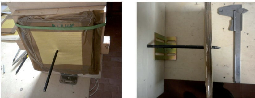
Figure 15. Pictures of a panel sample just after the ballistic test.
