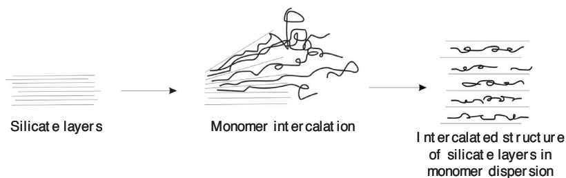
Figure 4. Intercalation of monomer, crosslinker and photoinitiator molecules between clay minerals silicate layers.
